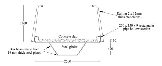
Figure 3. Cross-section of bridge deck (all dimensions in mm).
