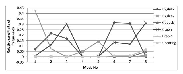
Figure 12. Sensitivity of modal frequencies to selected updating parameters.
