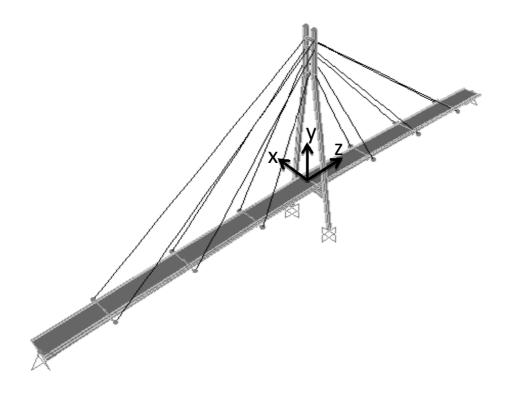
Figure 11. FE model of the bridge.
