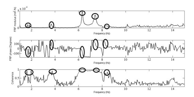
Figure 8. FRF measured during vertical shaker test.
