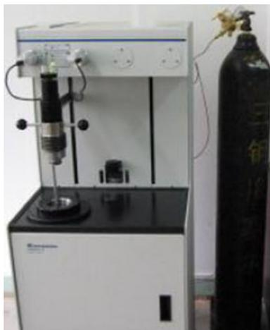
**Fig. 3** Micro-Meritics automatic mercury intrusion apparatus (Auto-Pore IV)
