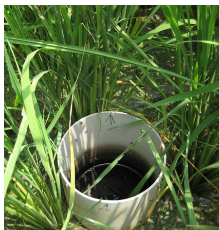
Figure 1. Perforated tube inserted into the soil to measure the height of the water table in the rice field for AWD in Bangladesh.
