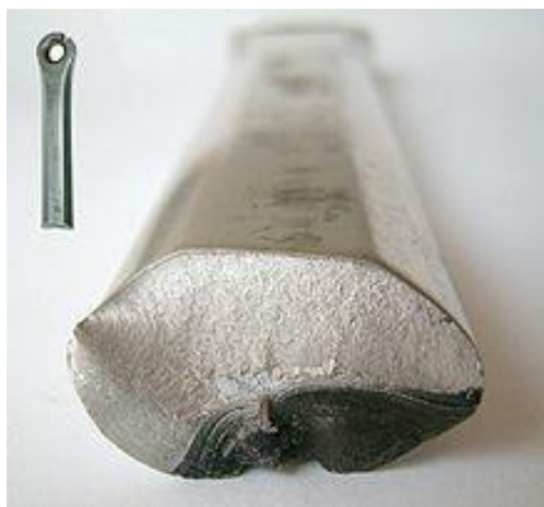
Figure 1 A failed connecting rod
