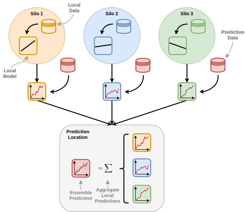
Figure 1: Visual depiction of the ensemble model sharing methodology. Each client trains a model on their own local data, then this model is evaluated on some prediction data, the resulting predictions are aggregated to produce a global prediction.
