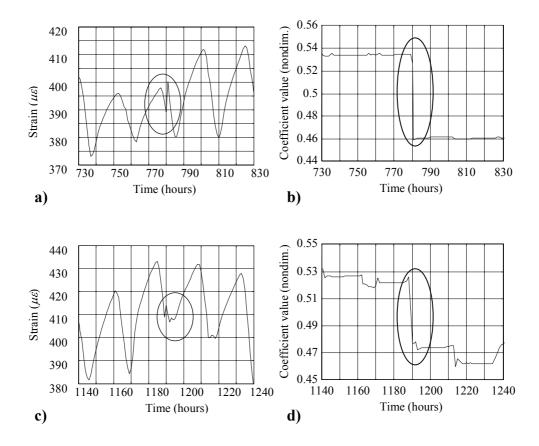
Figure 8. Time series of strains and values of coefficient  $\mathbf{A}_{t,1}$ : a) strains corresponding to tensioning event T24, b) values of coefficient  $\mathbf{A}_{t,1}$  corresponding to tensioning event T24, c) strains corresponding to unknown construction event, and d) values of coefficient  $\mathbf{A}_{t,1}$  corresponding to unknown construction event.
