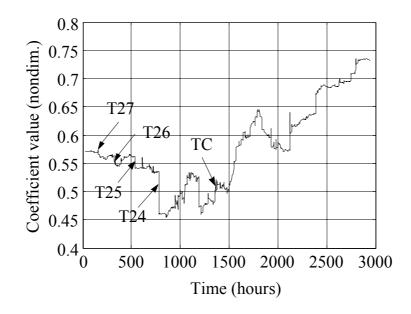
Figure 5. Identified values of first regular AR polynomial coefficient,  $\mathbf{A}_{t,1}$ , during bridge construction.
