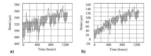
Figure 9. Strains recorded after construction: a) gauge SG31-1, and b) gauge SG23-1.
