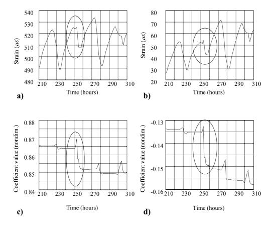
Figure 10. Time series of strains and values of ARIMA coefficients for a post-construction event: a) strains recorded by SG31-1, b) strains recorded by SG23-1, c) values of coefficient  $\mathbf{A}_{t,1}(1,1)$  d) values of coefficient  $\mathbf{A}_{t,1}(1,2)$ .
