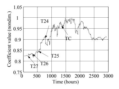
Figure 6. Identified values of first seasonal MA polynomial coefficient,  $\mathbf{C}_{t,1}^{(S)}$ , during bridge construction.
