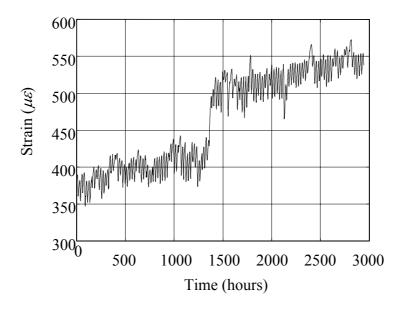
Figure 4. Strains recorded at gauge SG31-1 during construction and shortly after opening.
