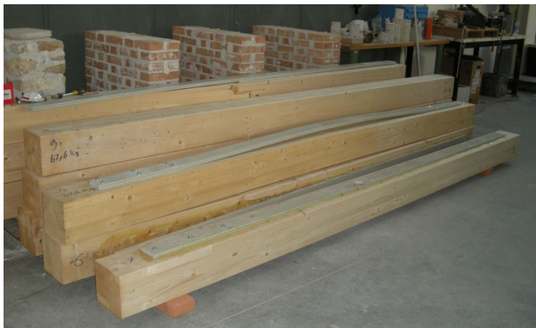
Figure 2: Hardwood a) and softwood b) beams before testing.
