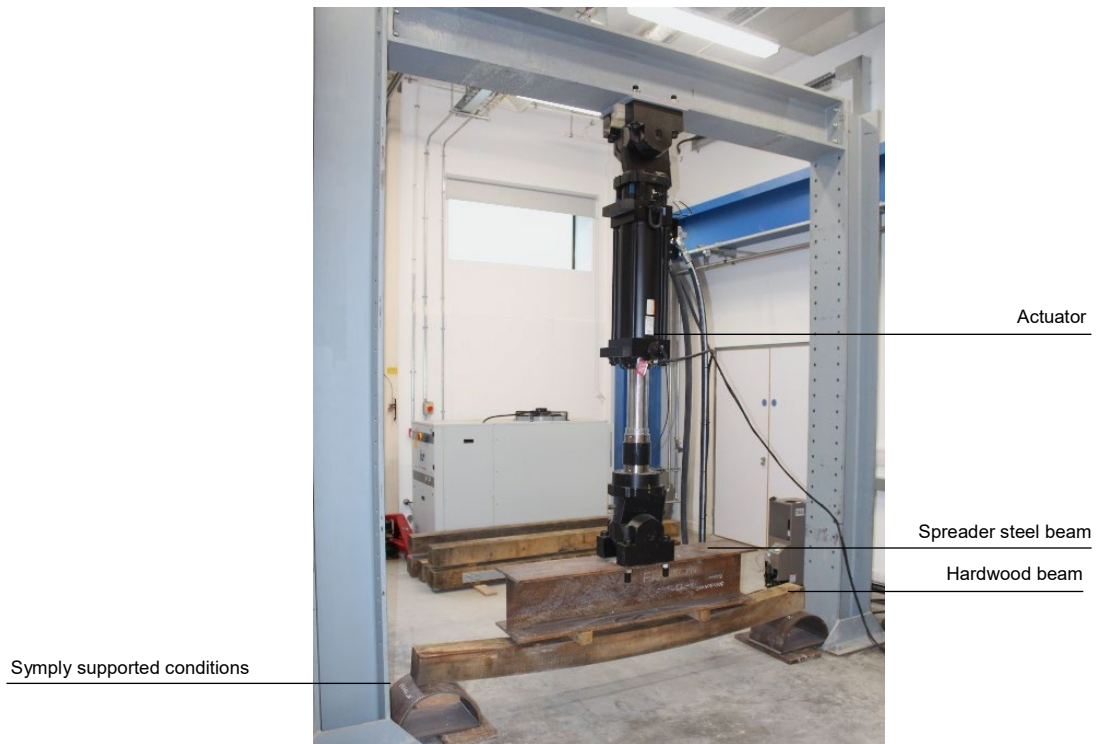
Figure 8: Bending test of hardwood beams.
