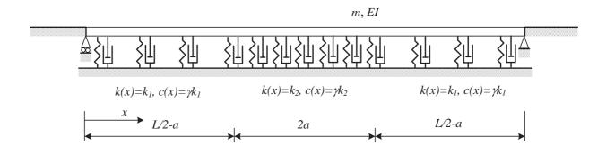
Fig. 5. Euler-Bernoulli beam on viscoelastic foundation in Example 2.
