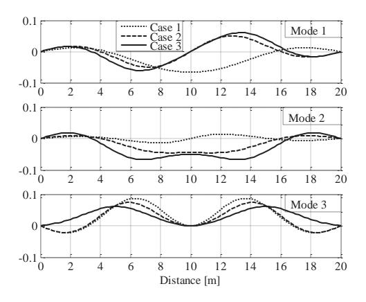
Fig. 7. Imaginary part of the first three continuum right mode shapes in Example 2.
