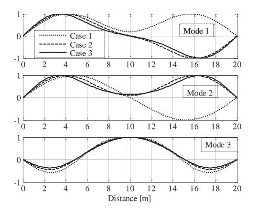
Fig. 6. Real part of the first three continuum right mode shapes in Example 2.
