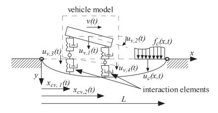
Fig. 1 Interaction of 1D continuum and moving MDOF oscillator.
