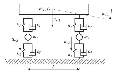
Fig. 2 Four-degree-of-freedom vehicle model.
