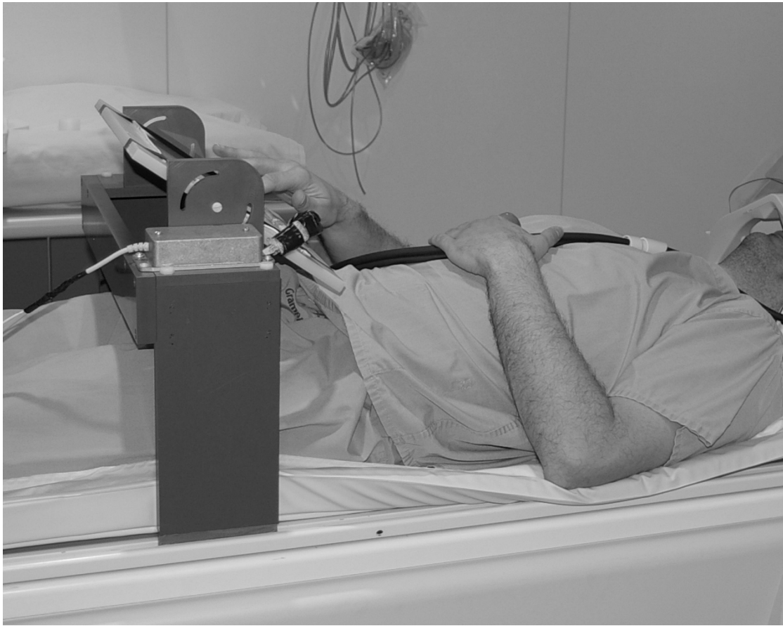
Fig. 1. Touchscreen in-situ showing acrylic chassis and tilting mechanism
