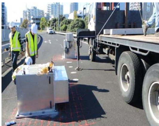
Figure 5. Eccentric mass shakers mounted on the bridge.
